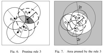
PRUNING RULE 3: If  $mindist(R_{cnd}, o_i) > 2r$  for any internal guard object  $o_i$  then no object in  $R_{cnd}$  can affect the safe zone.
