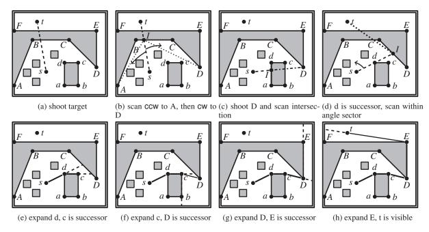
Figure 2: RAYSCAN Example - The dashed line is a ray shot, it turns dash dot line after intersecting with a polygon. Each corner scanned by RAYSCAN is shown by a dotted line from s to the corner. The solid lines are edges on the shortest path.
